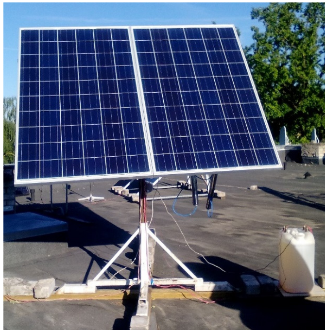
Fig. 1. Tracking device with two solar panels and water container
